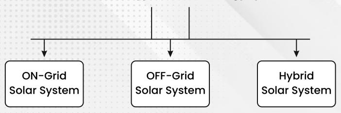
ON-Grid solar system: An ON grid solar system is a system that works along with the grid. This means that any excess or deficiency of power can be fed to the grid through net metering.
